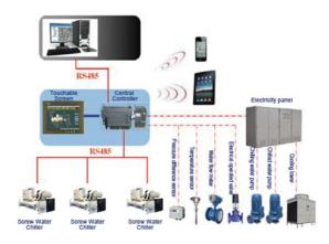
Fujiair water cooled screw chiller adopts a Microprocessor controller which enables the user to monitor and control the chiller with precise accuracy. The Microprocessor control system guarantees high precision and stability. The module-designed control system is easy for installation and maintenance. The chiller comes with a reserved RS485 port which can be interfaced with BAS (Building Automation system). Remote monitoring and control of the chiller is possible.
